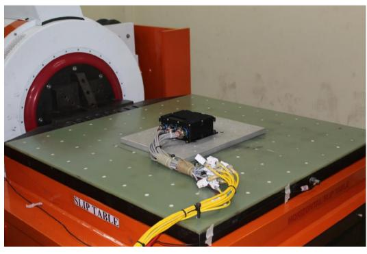
Functional Vibration and shock test - XX Axis
